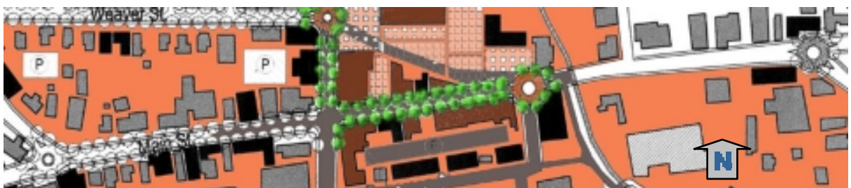
This diagram suggests how roundabouts at Main and Jones Ferry and Main and Rosemary could be situated.
